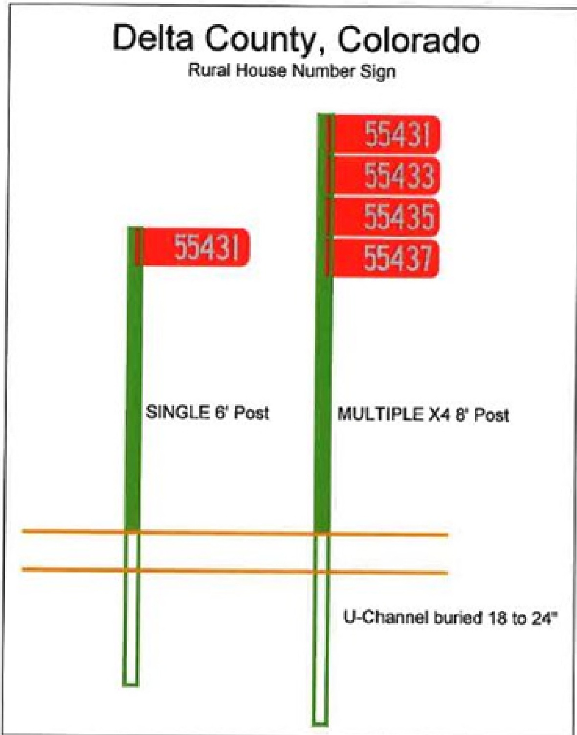
Figure 2 Delta County 9-1-1 Address Sign Installation Example
