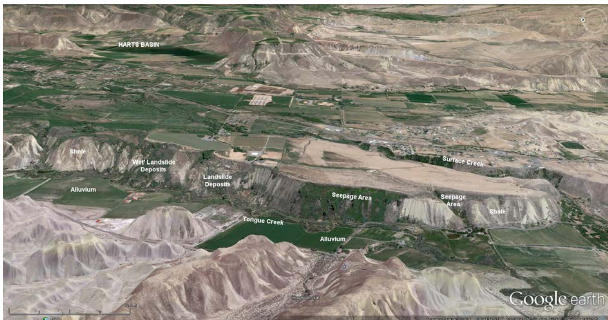
Figure 25e. Google Earth View of Detail of Central Part of the Valley Bottom Subsystem at Tongue Creek and Tributaries, Looking East. Note Seepage Faces and 'Wet' Landslide Deposits on Terrace Slopes.
